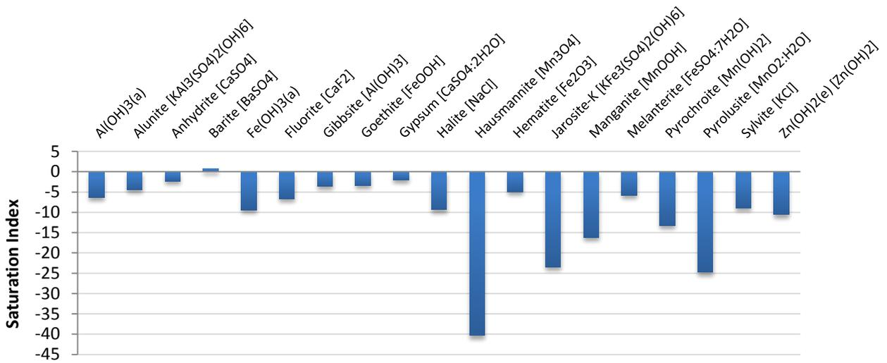
Figure 6 Saturation Indices of solid phases in pit lake water
