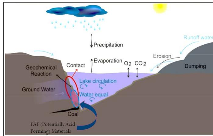
**Figure 5 Schematic of pit lake and AMD formation process**
