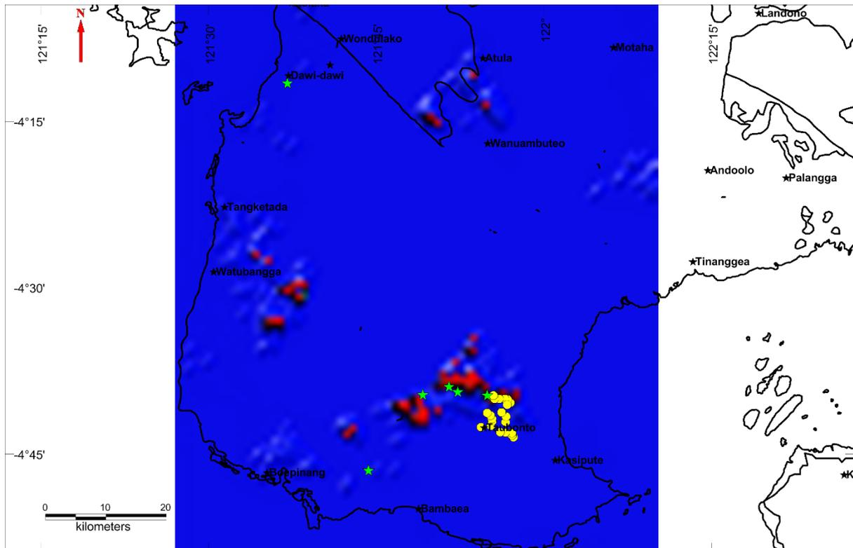
Figure 7: Sustainable prospectivity map for placer gold in the Bombana region of South East Sulawesi. The location of known gold occurrences (green stars) and geochemical sample points (yellow circles) are shown on the map. The red areas indicate zones of sustainable prospectivity for placer gold.
