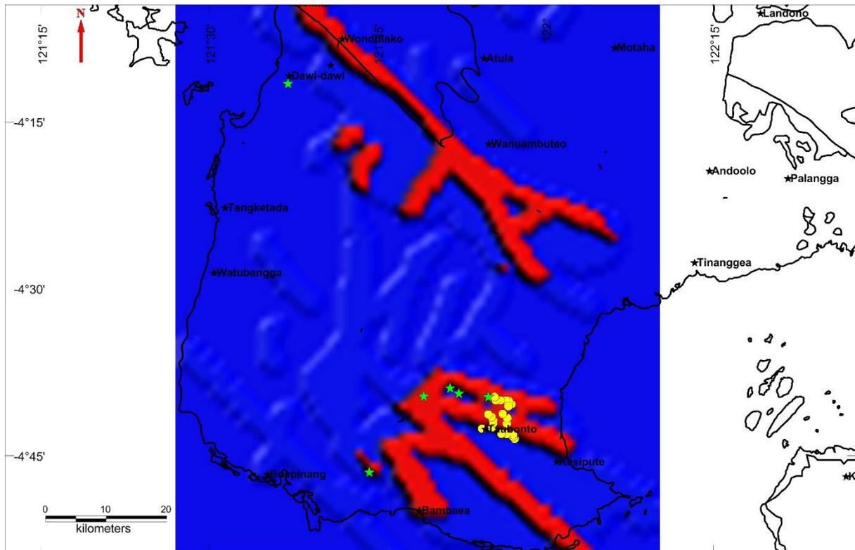
Figure 3: Orogenic gold prospectivity map for the Bombana region in South East Sulawesi using the parameters in Table 1. The location of known gold occurrences (green stars) and geochemical sample points (yellow circles) are shown on the map as a validation measure. The red areas indicate a higher prospectivity for orogenic gold.
