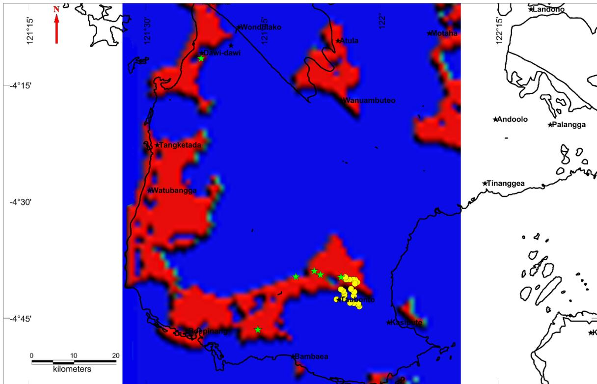
Figure 5: Sustainability map for South East Sulawesi using the parameters in Table 3. The location of known gold occurrences (green stars) and geochemical sample points (yellow circles) are shown on the map. The red areas indicate zones that are more favourable for exploration and mining based on sustainability criteria.
